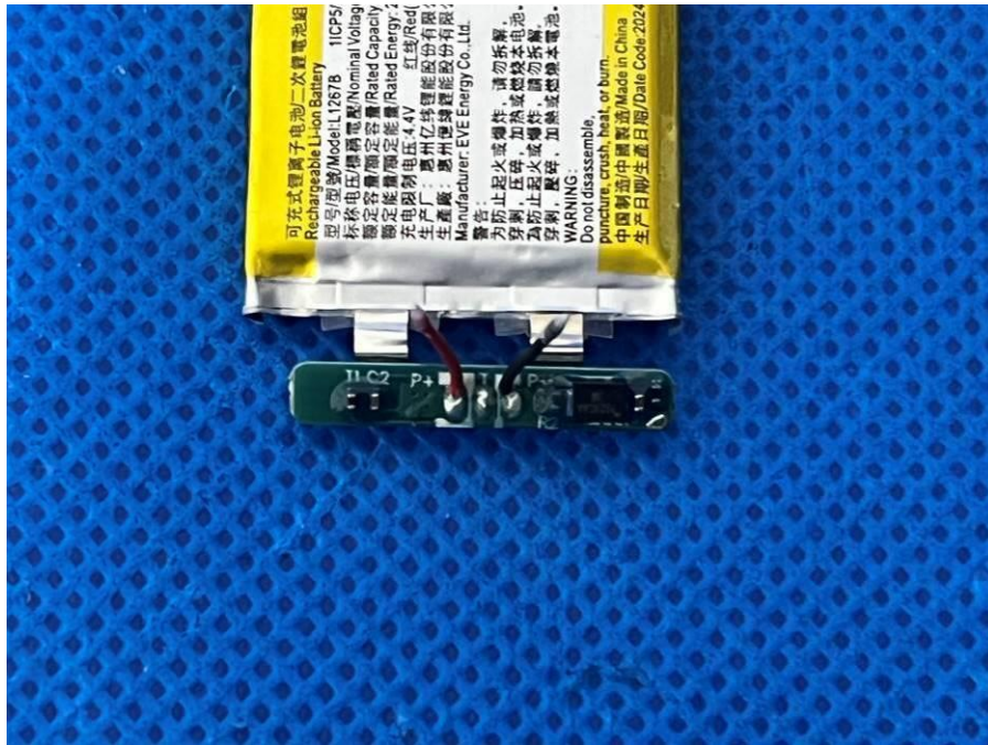
Figure 19: Protective board of charging case battery
